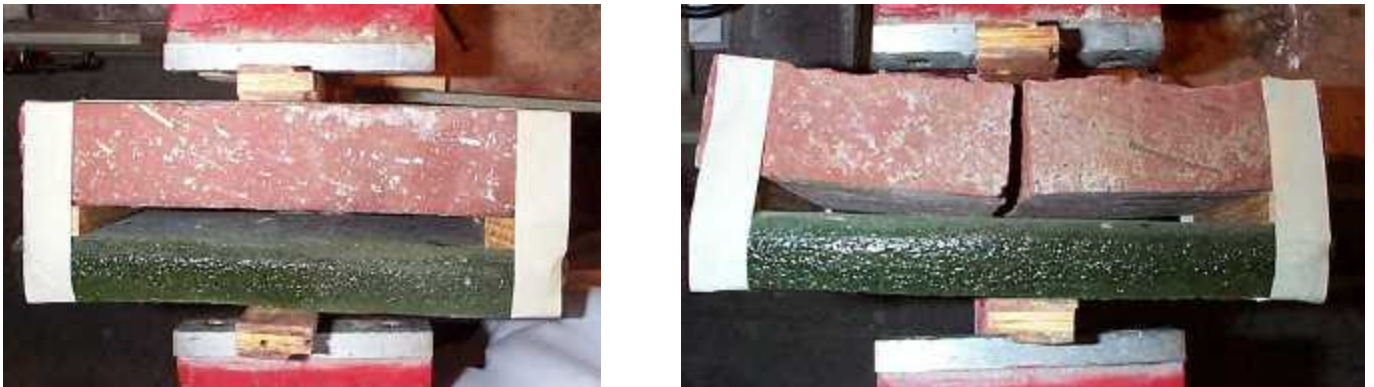
Figure 1 - 1600 gram clay brick and 1250 gram glass brick before & after breaking
