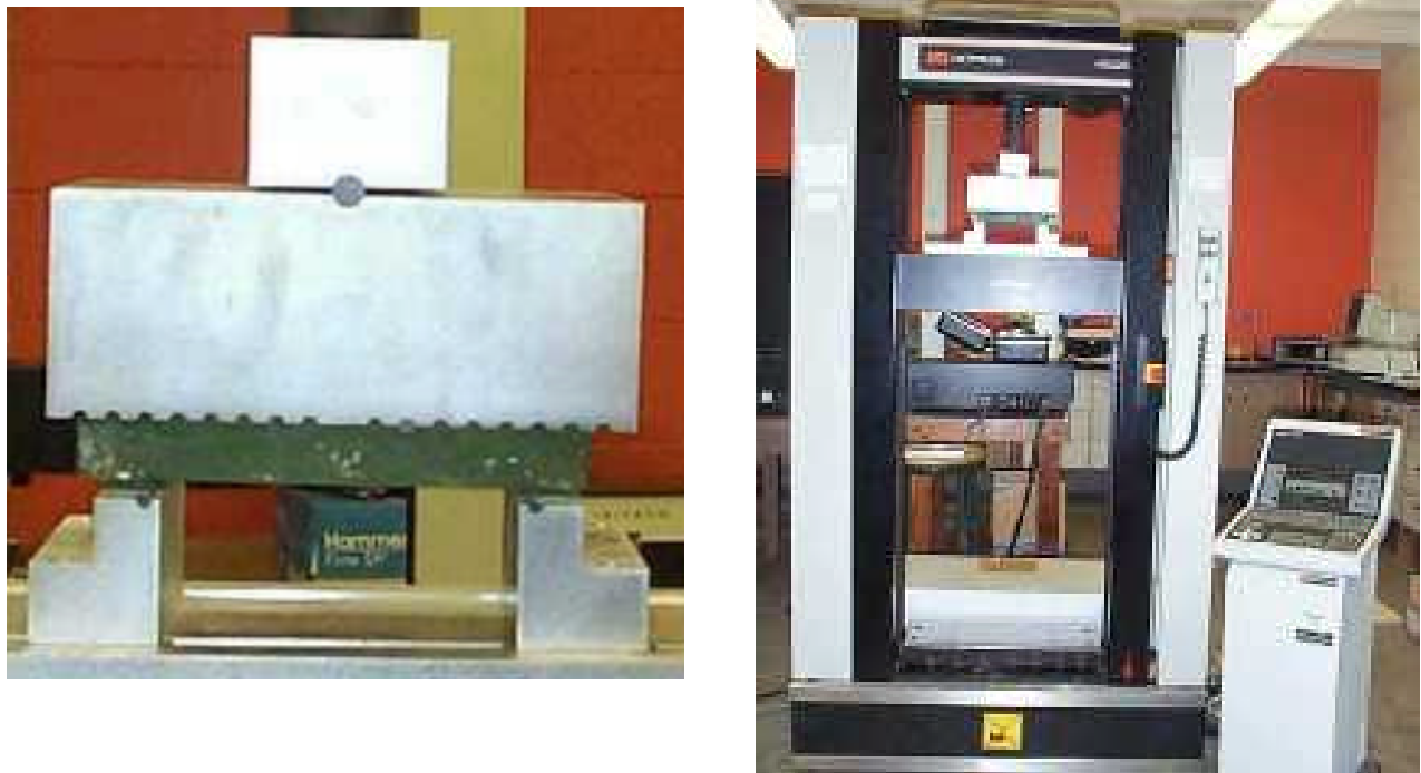
Figure 5 - Flexure Testing Fixture and Test Instrument
