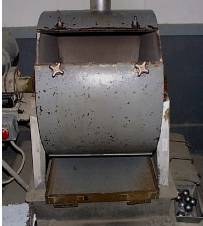
Figure 13. Los Angeles Abrasion test machine
