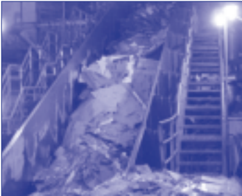
Recovered old corrugated containers are fed into the repulping process at Bay State Paper Company.
